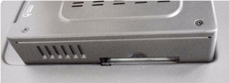
Figure 2.2: Install CompactFlash Memory Card
