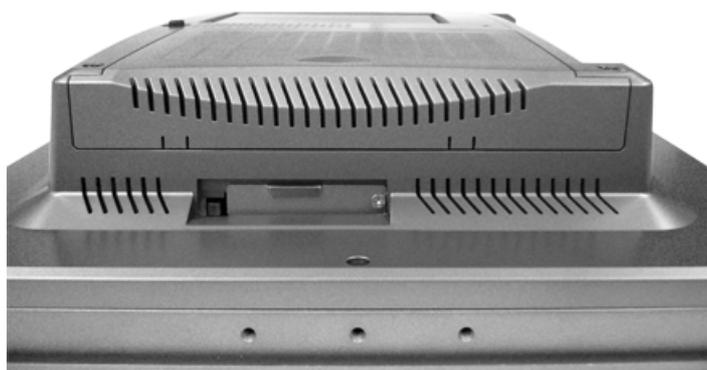
**Figure 2.2 Install CompactFlash Memory Card**
