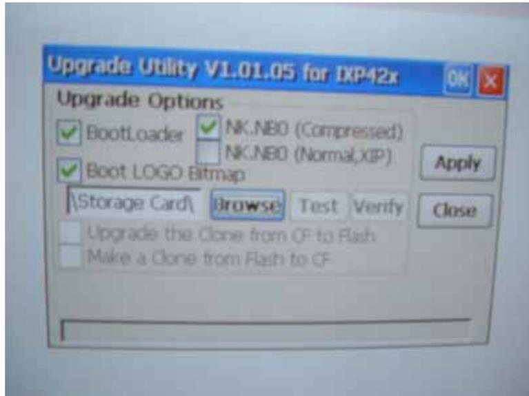
Figure 4.7 Press Apply button in order to upgrade onboard flash ROM After the upgrade process done, reboot system..
