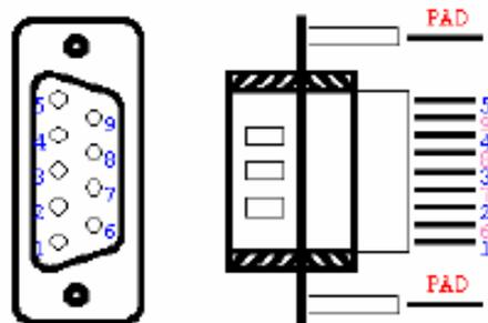
Figure 3.1 COM1 (RS-232) serial port
