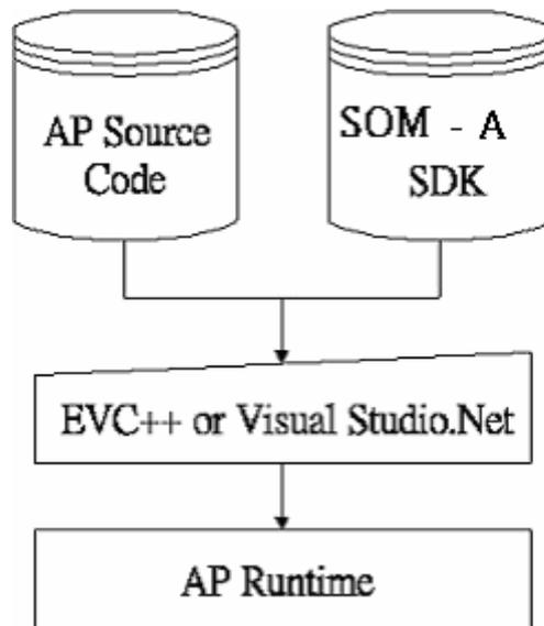
Figure 4.16 Flow-chart of Building Windows<sup>®</sup> CE.NET runtime
