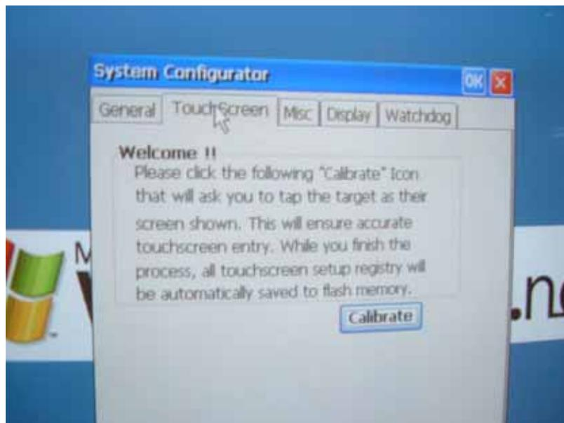
Figure 4.9 Touch-screen calibration
