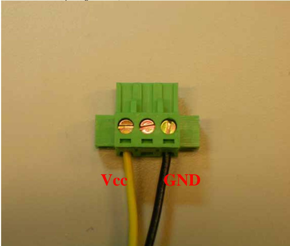
4. Plug the male power connector into female power connector in SPC.
