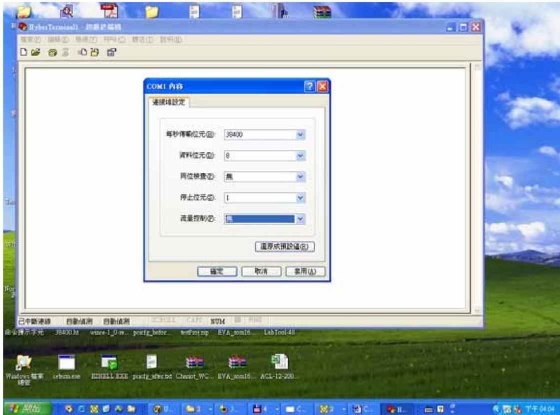
Figure 4.5 Configure COM port parameters
