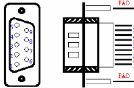
Figure 3.2 COM2 (RS-232) serial port
