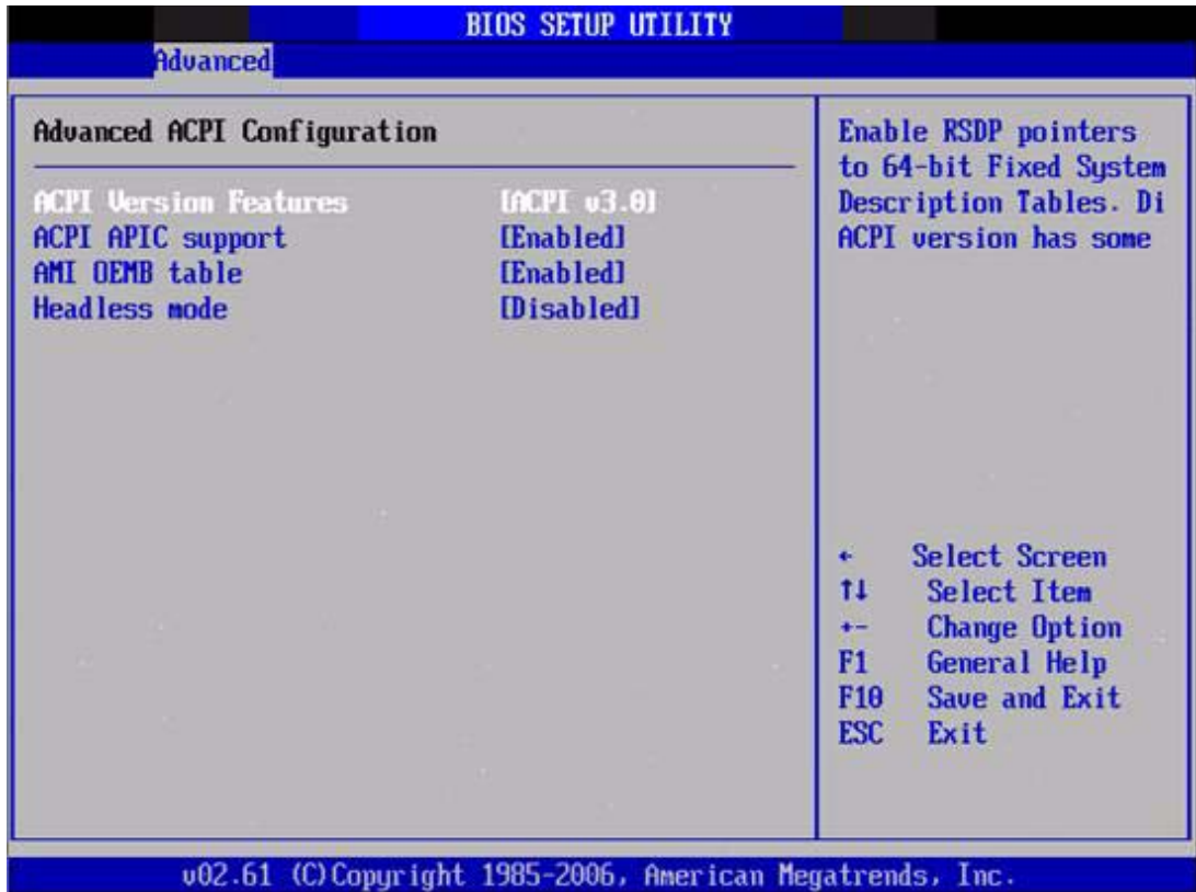
Figure 3.10 Advanced ACPI Configuration
