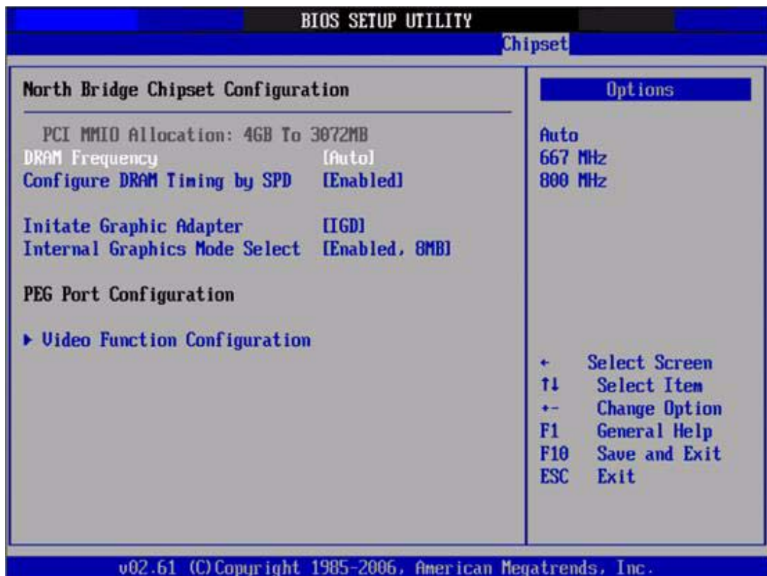
Figure 3.25 North Bridge Configuration
