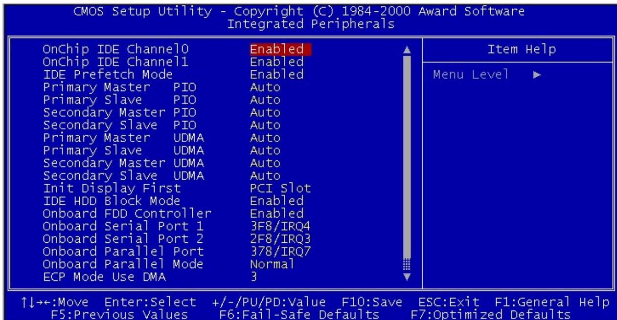
**On-Chip IDE Channel 0 [Enabled/Disabled]:** The system provides an onboard on-chipset PCI IDE controller that supports Dual Channel IDE. A maximum of 4 IDE devices can be supported.
