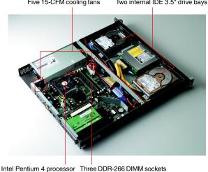
Two USB ports VGA port COM 2 LAN 1 Power supply Two PS/2 COM 1 LAN 2 ports
