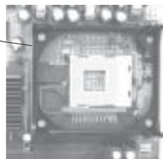
3. Place a retention bracket in the proper position and secure it by pressing two pegs into the retention holes until you hear a \*click\*. The clicking sound indicates that the peg is locked and secured.
