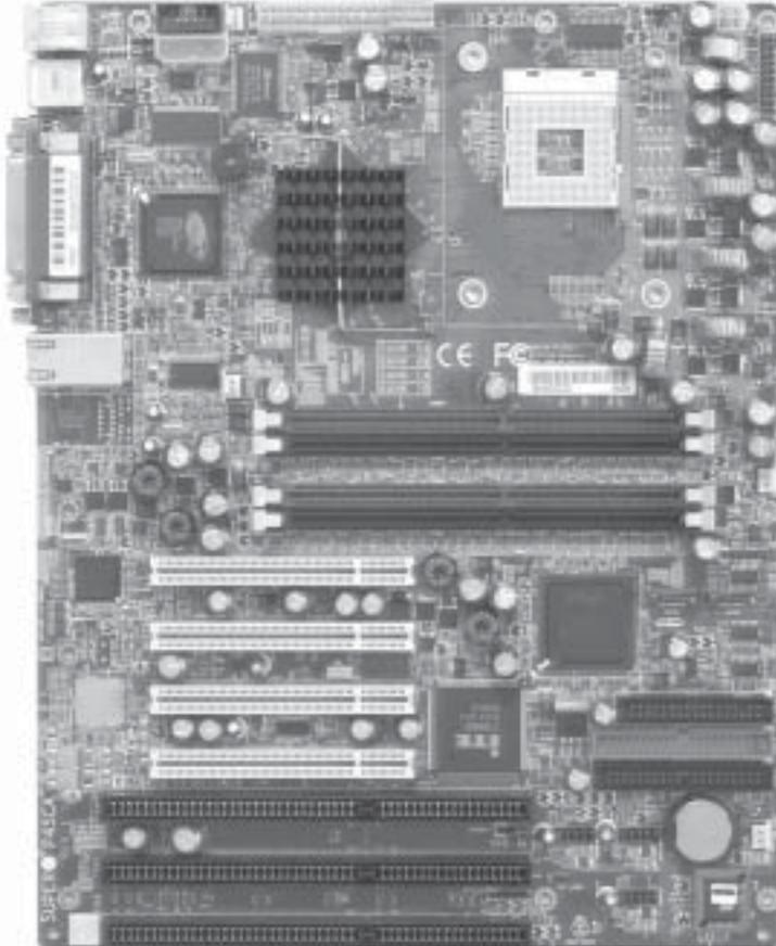
**Figure 1-2. SUPER P4SCA Motherboard Layout**
