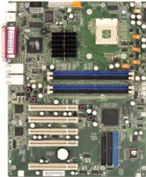
Figure 1-4. SUPER P4SCE Motherboard Layout
