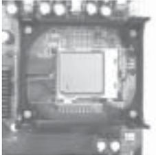
6. Install the CPU in the socket. Make sure that Pin 1 of the CPU is seated on Pin 1 of the socket (both corners are marked with a triangle).
