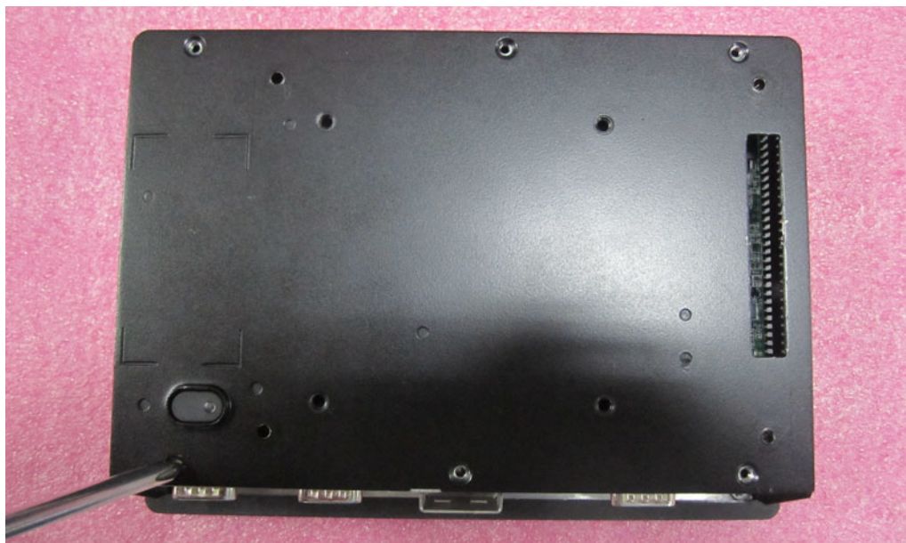
Figure 4.2 Unfastening the Rear Cover
