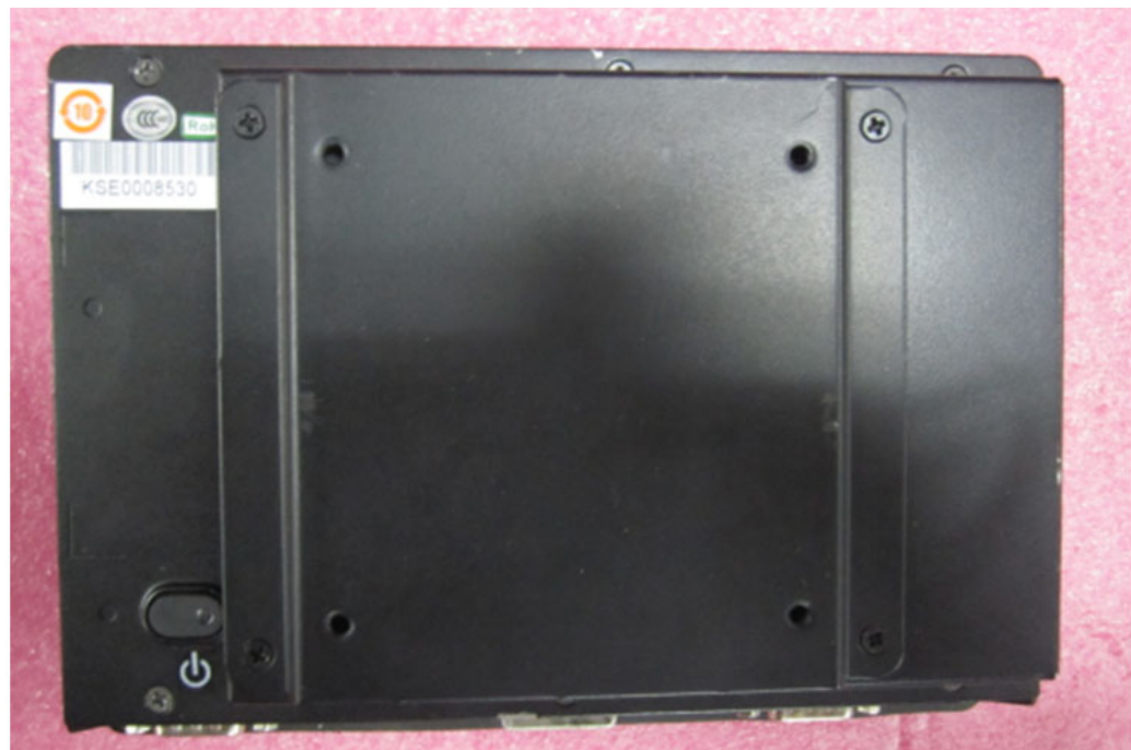
Figure 4.5 HDD Module is Mounted to the Machine
