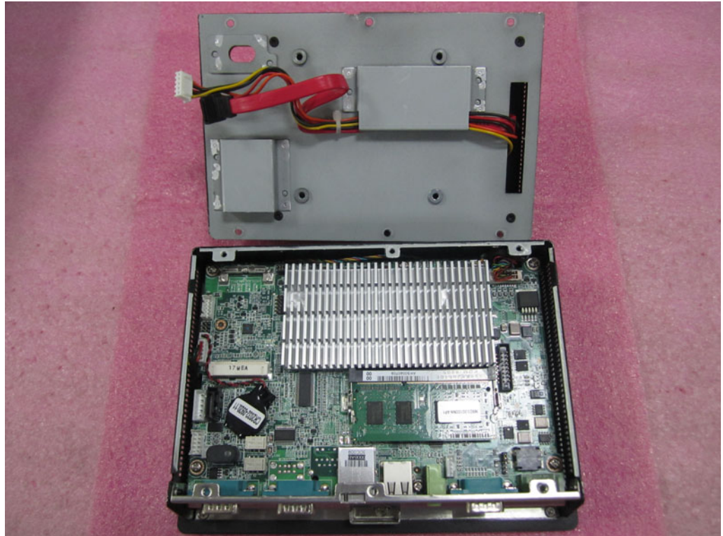
Figure 4.4 Assembly HDD Module to Rear Cover
