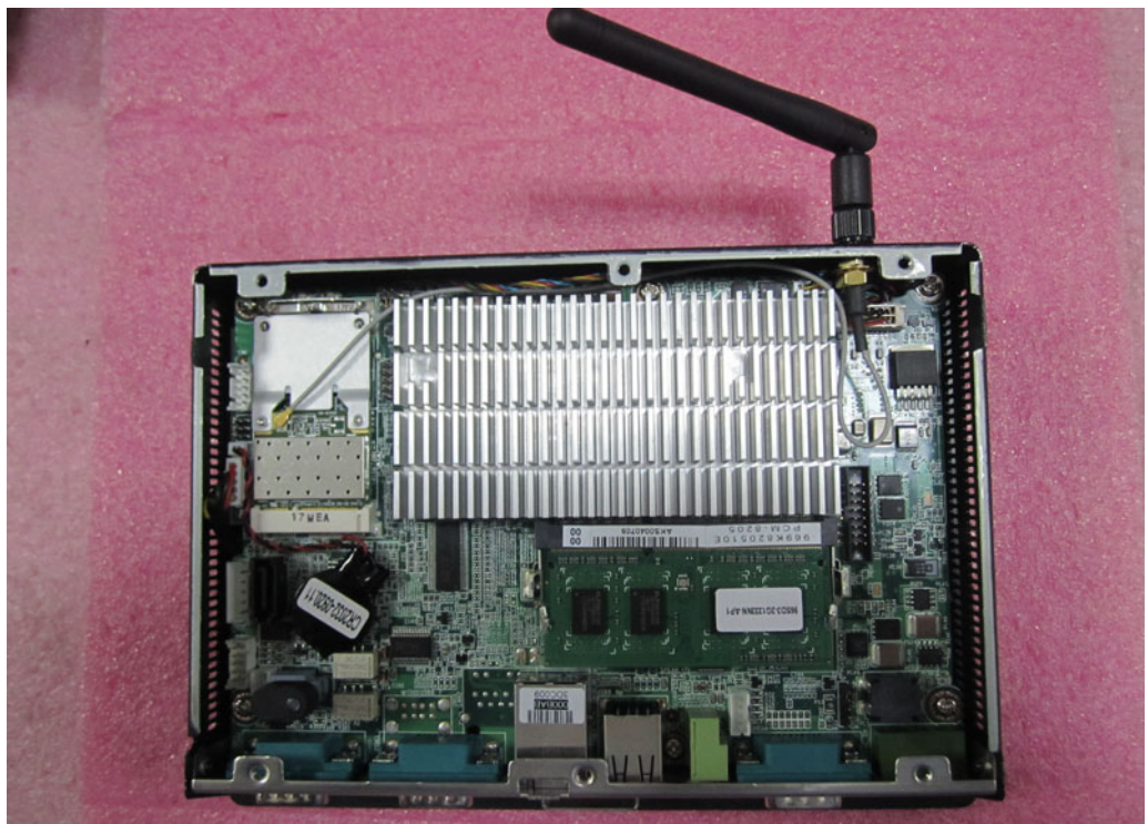
Figure 4.8 Install the wireless LAN card and antenna
