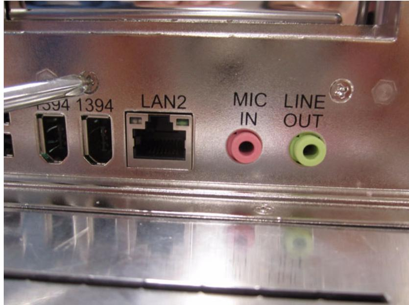
**Figure 4.10 Fasten Screw on IO Shielding**
