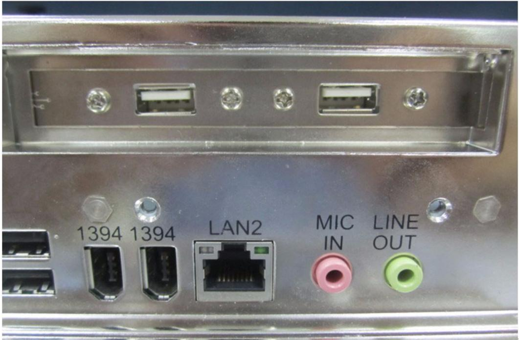
**Figure 4.21 Completed Assembled Dual-USB Cable**
