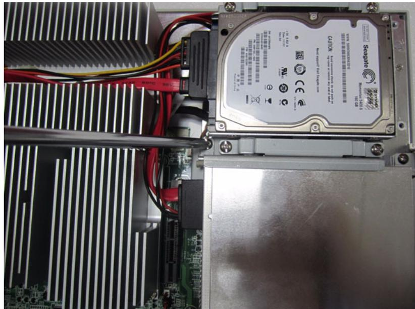
**Figure 4.11 Fasten Screws on the ODD Bracket**
