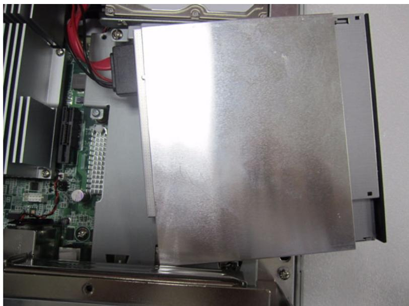
Figure 4.9 Plug in the SATA ODD Cable
