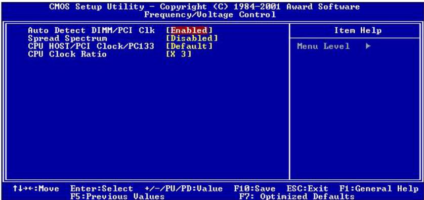
**Figure 3-9: Frequency/Voltage Control**
