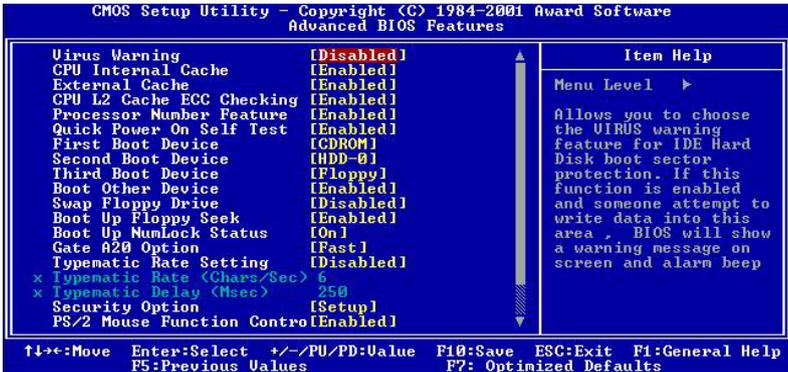
Figure 3-3: Advanced BIOS Features setup screen
