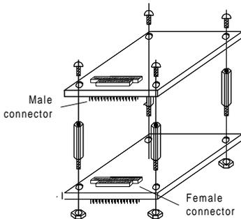
2. Screw the PCM-3612 to the brass spacer.
