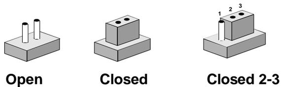
The jumper settings are represented in this manual with the following diagrams:
