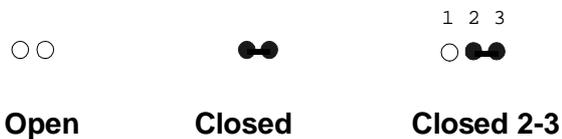
A pair of nonmagnetic, needle-nosed pliers may be helpful when working with jumpers. In order to prevent an unused jumper from getting lost, you may leave it inserted on a single jumper pin.
