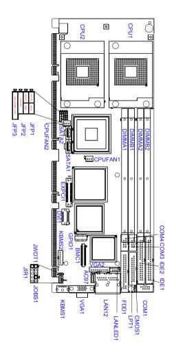
**Board Layout: Jumper and Connector Locations**
