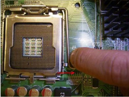
Step 2. Align the triangular marking on the processor with the cut edge of the socket.
