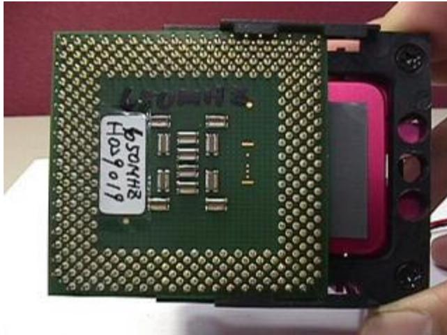
Figure 3-3: Pushing the Coppermine/Celeron™ into the frame
