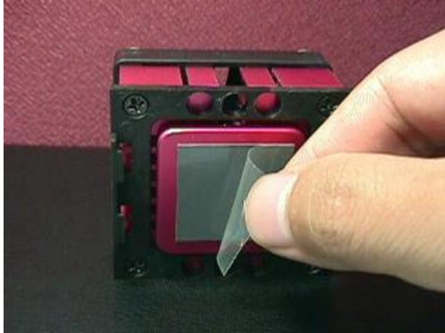
Figure 3-2: Peeling off the thin plastic coating of the CPU fan
