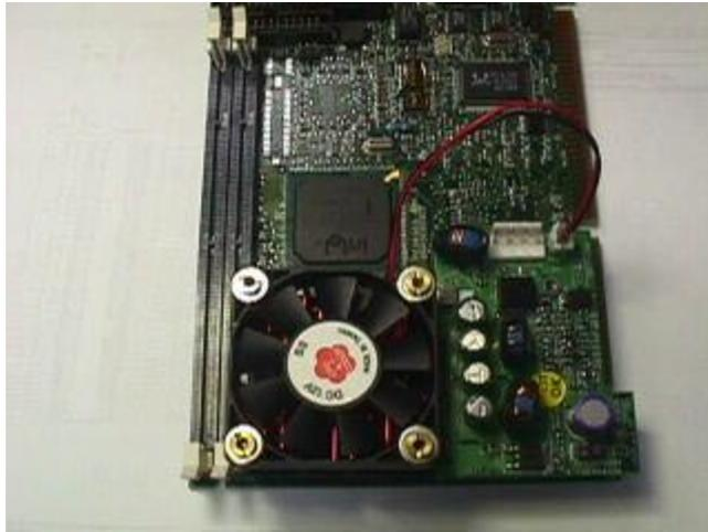
Figure 3-5: Affixing the CPU/fan assembly to the board
