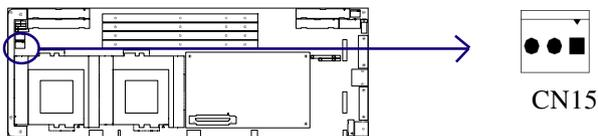
This connector supports cooling fans of 2 A or Less
