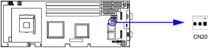
Connect to the CN1 on the Advantech backplane to enable the ATX function, 5V stand-by.
