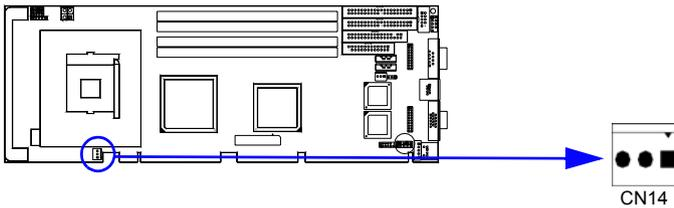
If fan is used, this connector supports cooling fans of 500mA (6W) or less.
