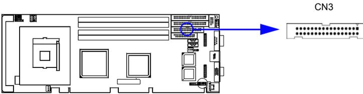
You can attach up to two floppy disk drives to the PCA-6187's on board controller. You can use 3.5" (720 KB, 1.44 MB) drives.
