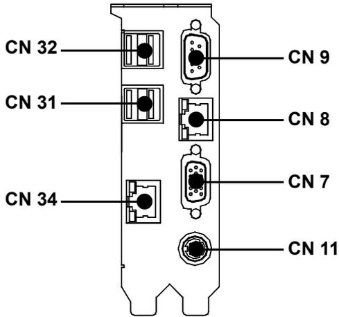
*Figure 1.2: I/O Connectors*
