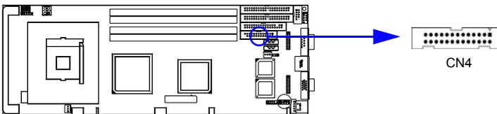
The parallel port is normally used to connect the single board computer to a printer. The PCA-6187 includes an onboard parallel port, accessed through a 26-pin flat-cable connector, CN4. The card comes with an adapter cable which lets you use a traditional DB-25 connector. The cable has a 26-pin connector on one end and a DB-25 connector on the other, mounted on a retaining bracket. The bracket installs at the end of an empty slot in your chassis, giving you access to the connector.
