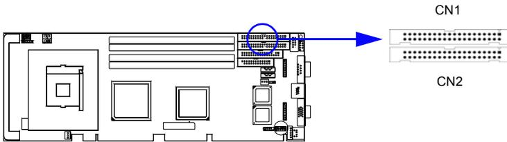
You can attach up to four IDE (Integrated Drive Electronics) drives to the PCA-6187's built-in controller. The primary (CN1) and secondary (CN2) connectors can each accommodate two drives.
