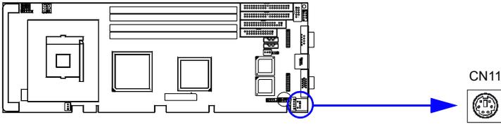
Two 6-pin mini-DIN connectors (CN11 and CN33) on the card mounting bracket provide connection to a PS/2 keyboard and a PS/2 mouse, respectively. CN11 can also be connected to an adapter cable (P/N: 1700060202, available from Advantech) for connecting to both a PS/2 keyboard and a PS/2 mouse.
