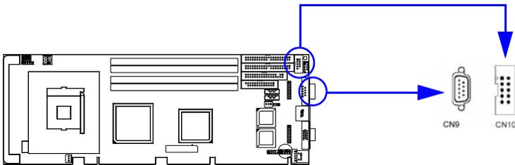
The PCA-6187 offers two serial ports, CN9 as COM1 and CN10 as COM2. These ports can connect to serial devices, such as a mouse or a printer, or to a communications network.
