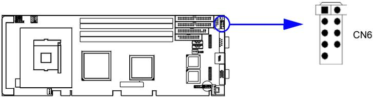
The PCA-6187 provides up to six ports of USB (Universal Serial Bus) interface, which gives complete Plug & Play and hot swapping for up to 127 external devices. The USB interface complies with USB Specification Rev. 2.0 support transmission rate up to 480 Mbps and is fuse-protected. The USB interface can be disabled in the system BIOS setup.
