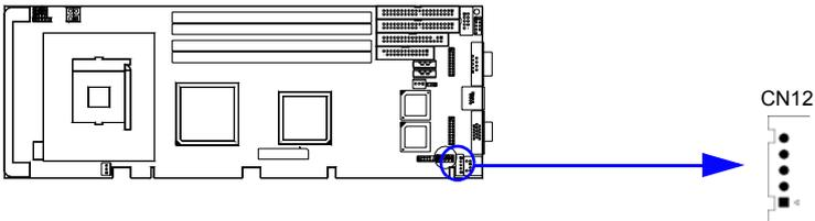
In addition to the PS/2 mouse/keyboard connector on the PCA-6187's rear plate, there is also an extra onboard external keyboard connector. This gives system integrators greater flexibility in designing their systems.
