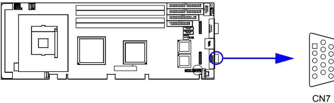
The PCA-6187 includes a VGA interface that can drive conventional CRT displays. CN7 is a standard 15-pin D-SUB connector commonly used for VGA. Pin assignments for CRT connector CN7 are detailed in Appendix B.
