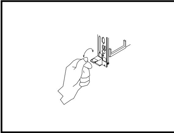
**Figure 2-5: Installing the card into the chassis**
