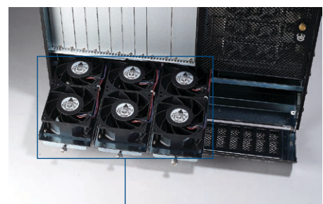
Six 80-CFM front-access hot-swappable fan modules
