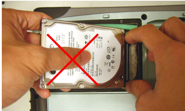
Figure 4.6 Incorrect removal of the HDD
