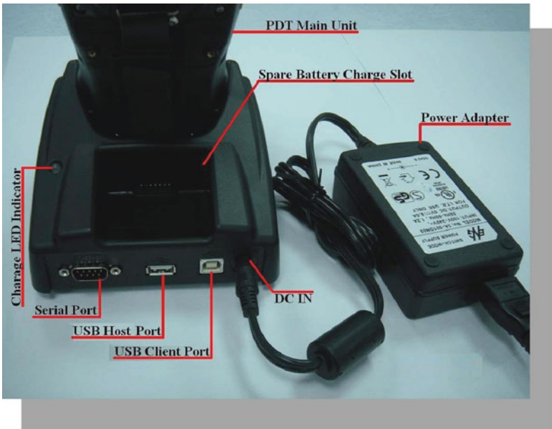
Figure 2.9: Charging with a Single Dock
