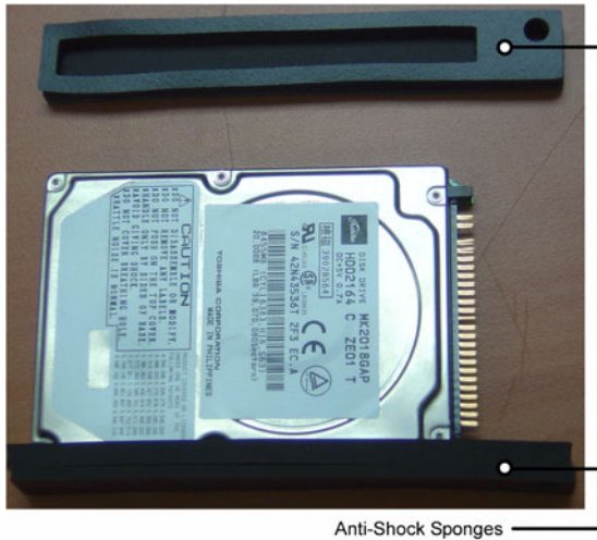
Figure 2.8: Adding Anti-shock Sponges to the HDD
