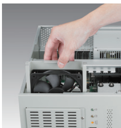
Easy-to-maintain cooling fan
