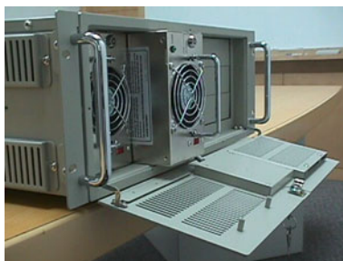
Figure 3-5: Replacing the redundant power supply module
