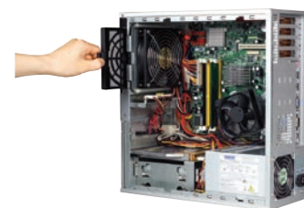
Gently press the hook to pull the air filter out
