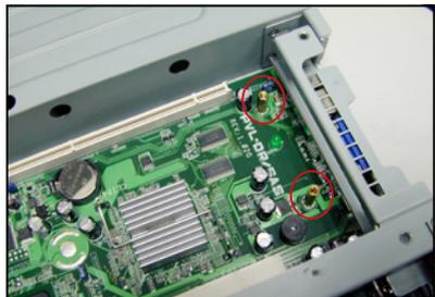
6. Insert the transfer card with the installed ZCR card into the transfer card slot on the system board.
