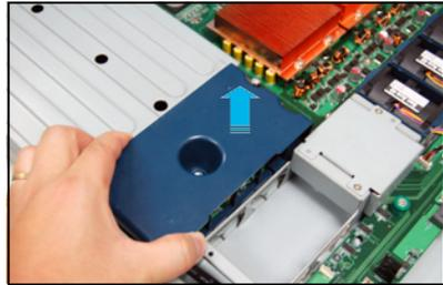
6. Using a screw driver to remove the screw on the back of the power backplane board, then remove the PSU power backplane board.
