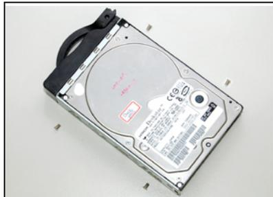
5. Carefully insert the drive tray and push it all the way to the depth of the bay until just a small fraction of the tray edge protrudes.
