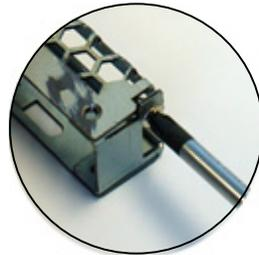
3. Insert a PCI-X card into the slot of the riser card, then put the screws back and fasten it.
