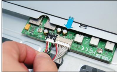
7. Disconnect the optical drive cable and power cable.
