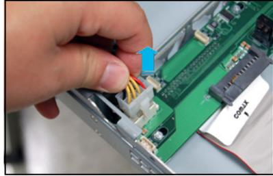
4. Push the power backplane board as shown until it is completely removed from the motherboard.
