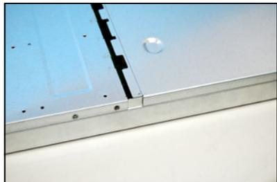
5. Push the front side of the top cover panel forward and lift it to expose the cable connectors and slots underneath.
