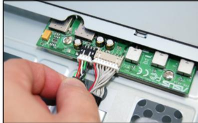
7. Disconnect the cable and power cable of the optical drive.
