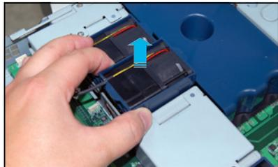
To install the device fan:
