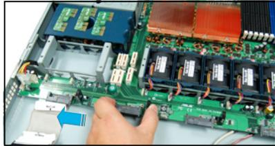
8. Remove the IDE cable and FPB/USB cable.
