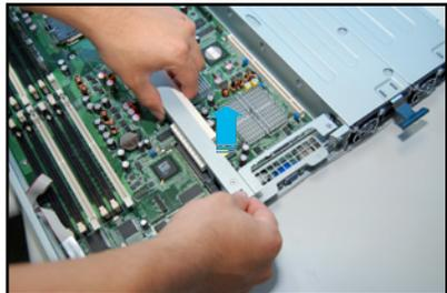
2. Prepare the SAS expansion module. connect it to the riser card and secure it.
