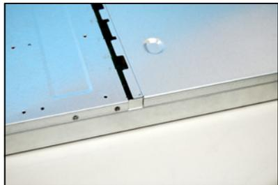
5. Lift the front side of the top cover panel to expose the cables connectors underneath.
