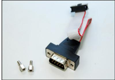
2. Open the top cover panel. Connect one end of the cable to the COM1 connector on the board, and then fit the other end into the COM1 opening of the rear panel.
