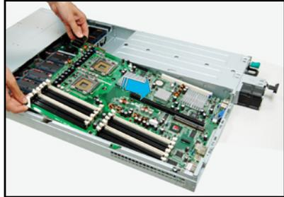
3. Match all the screw hole and secure the board to the chassis using the thirteen screws.
