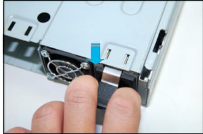
2. Pull the PSU outward and remove it.
