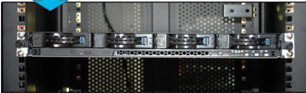
2. Tighten the two rack screws to secure the server to the rack.
