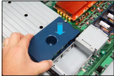
3. Push the power backplane board forward as shown until a slight sound indicates the board is firmly connected to the motherboard.
