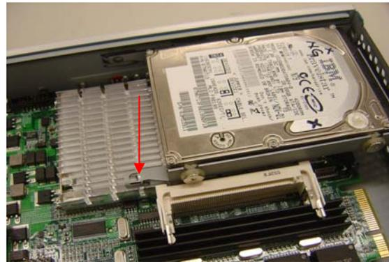
Figure 2-6: Install HDD
