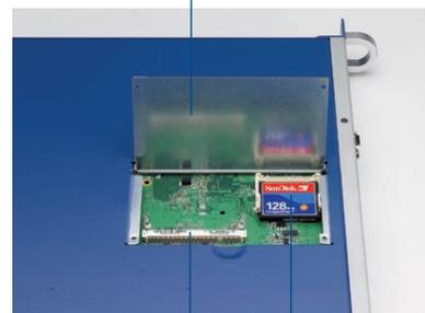
SDRAM socket CompactFlash socket
