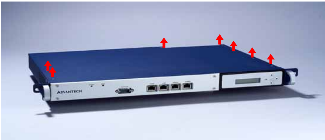
Figure 2-2: Removing the cover
