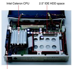
Two 5-CFM fans located next to the CPU for best ventilation
