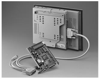
• Connectors: One MDR-26 connector for flat panel display One DB-15 connector for CRT monitor
