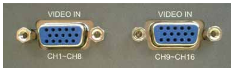
Figure 2.3: Video Input Connectors
