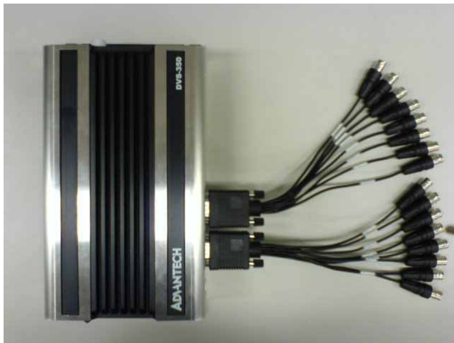
Figure 2.3: Video Input Connectors
