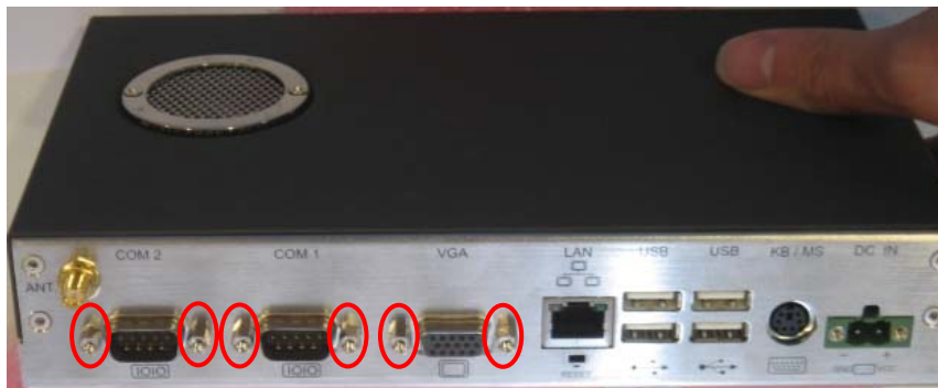
Figure 3.5: The back I/O side of DSA-3400
