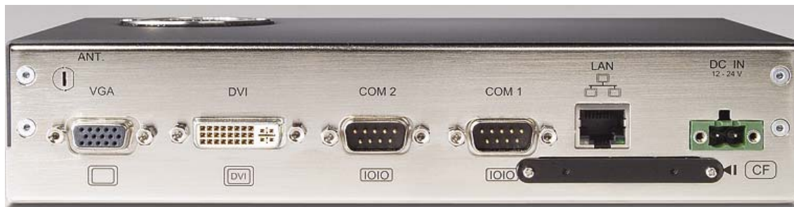
Figure 2.2: DSA-3400 rear metal face plate I/O connectors
