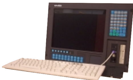
Figure 2-9: Connect front keyboard
