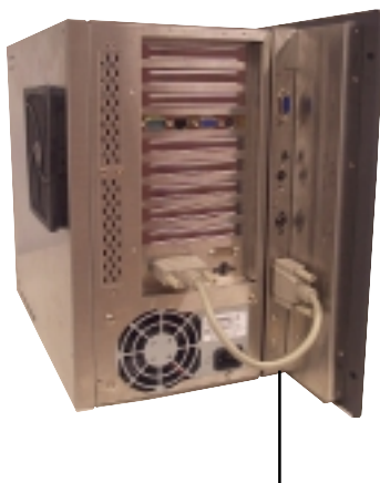
Connect USB/Indicator/Power cable to chassis
