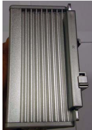
Figure 3.7: R DIN Rail Mounting Module on ARK-3381
