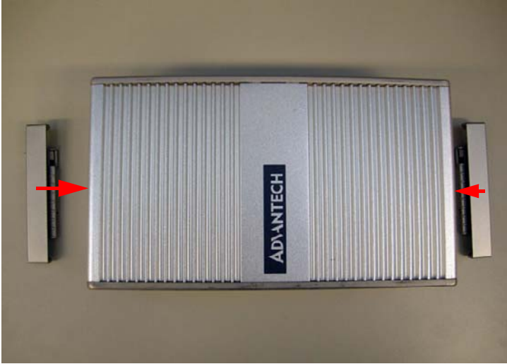
Figure 3.6: DIN Rail Mounting Module orientation
