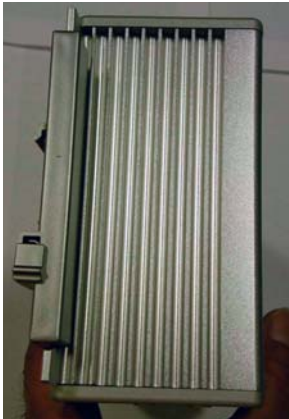
Figure 3.7: L DIN Rail Mounting Module on ARK-3381
