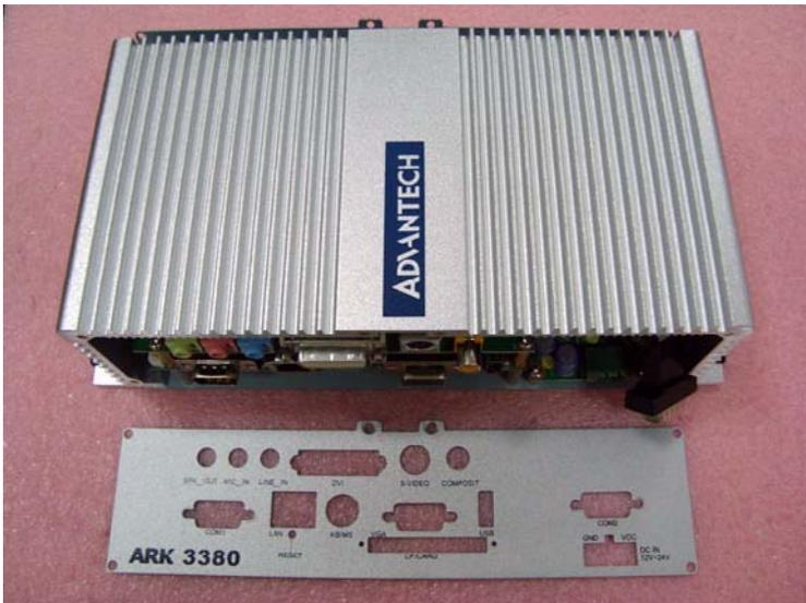
13. The system after the top cover has been removed.
