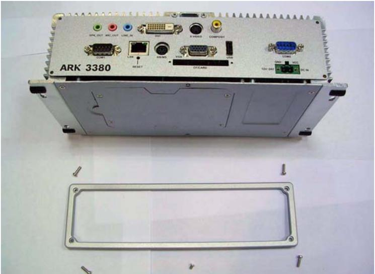
10. Unscrew the 2 screws which are located on the Rear Metal Face plate.
