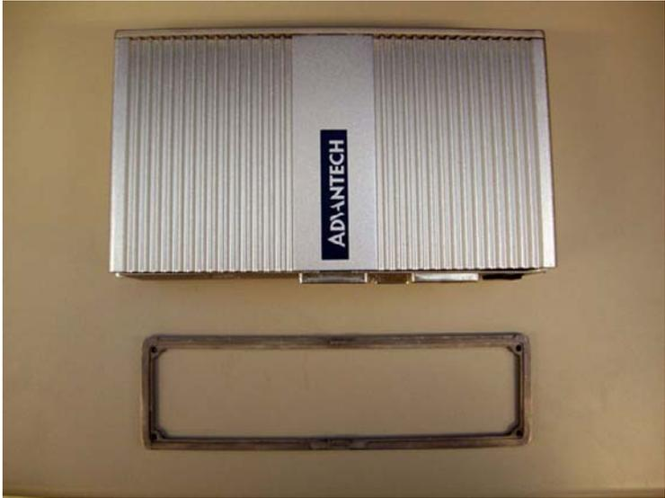
5. Unscrew the 2 screws which are located on the Front Metal Face plate.
