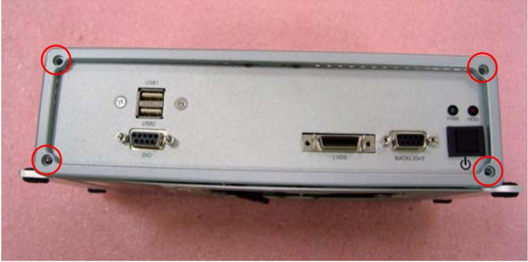
3. Remove the front frame bracket by carefully pulling and lifting the bracket in order to unlock it.
