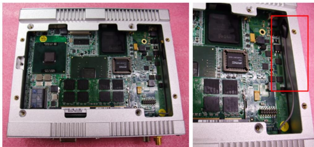
**Figure 5.11 UMTS/HSDPA SMA cable internally**
