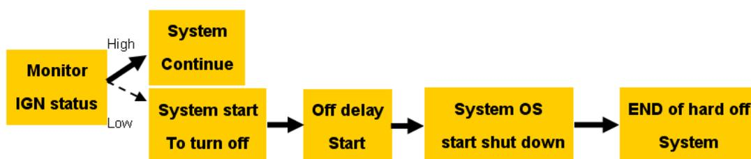
Figure 4.3 Turn off procedure of PIC firmware
