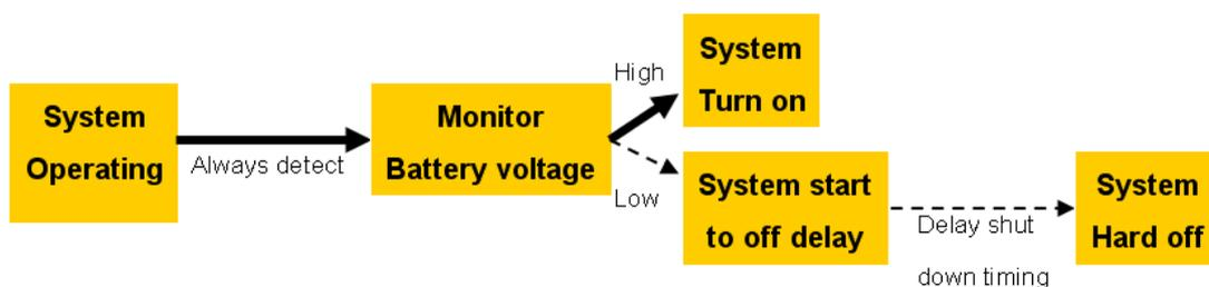
Figure 4.5 Battery status checking of PIC firmware
