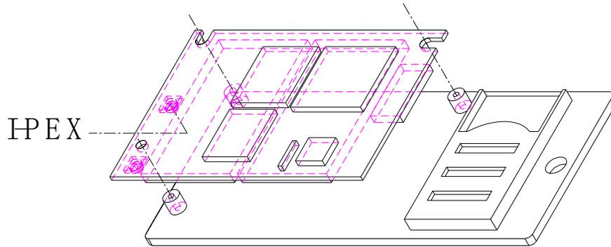
**Figure 5.9 install Siemens module on AMO board**
