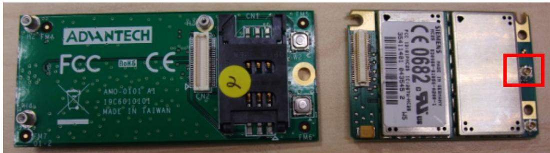
**Figure 5.10 AMO-EDGE base board and Siemens module**
