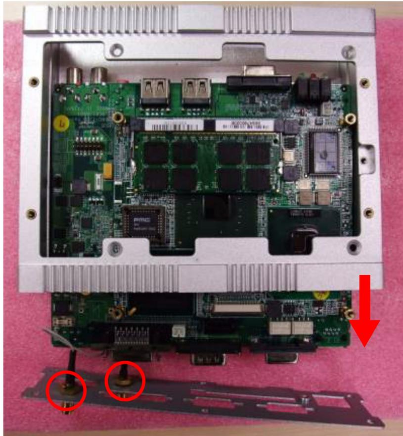
10. Take off the internal cable connector from the WLAN module and GPS antenna connector.
