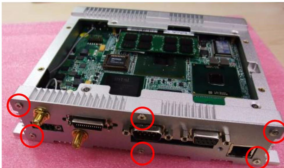
8. Unscrew the screws and hex-bolts in the middle of the rear panel.
