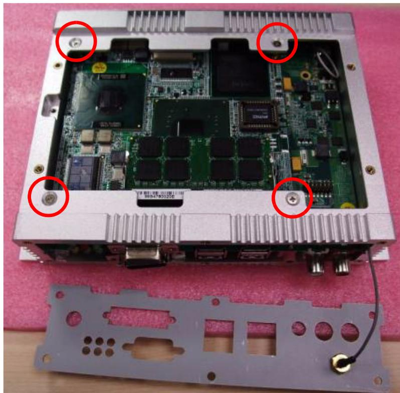
7. Unscrew the six screws on the rear panel.
