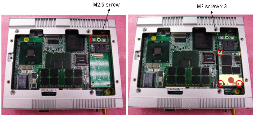
**Figure 5.13 Installation AMO-HSDPA on ARK-1388V**
