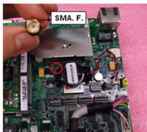
2. Insert the board on top side and screw the four screws on top side.
