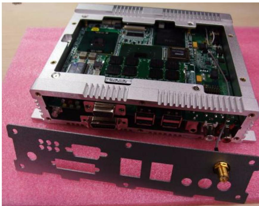
5. Put on the front IO plate and screw the LVDS connector first, then screws the screws on the front plate
