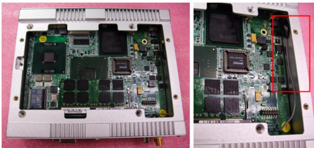
**Figure 5.4 GPRS/EDGE SMA cable internally**
