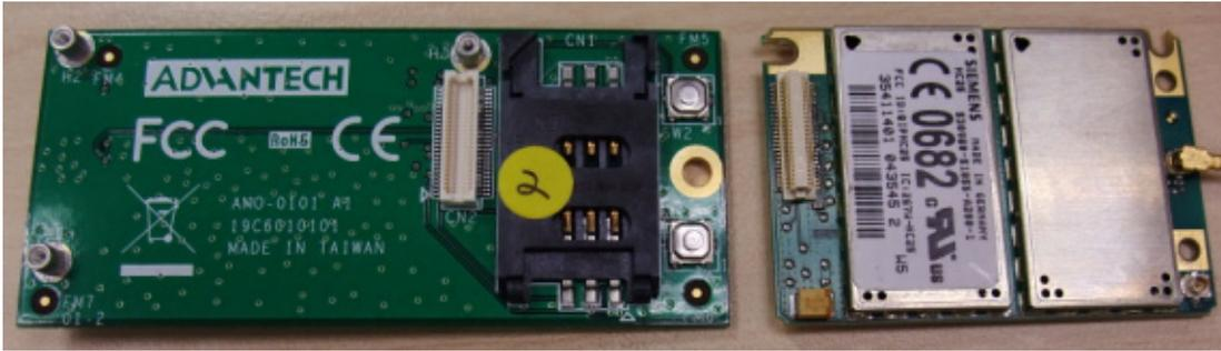
**Figure 5.12 Siemens antenna connector**
