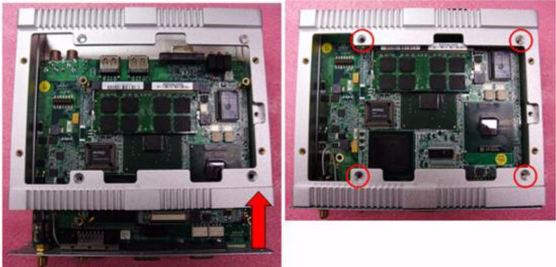
3. Screws the screws on the rear plate.
