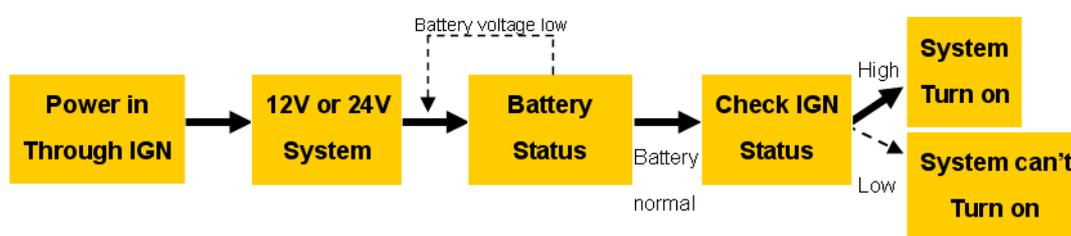
Figure 4.2 Turn on procedure of PIC firmware
