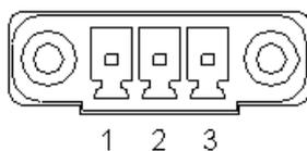
Figure 2.15 Power Input Connector
