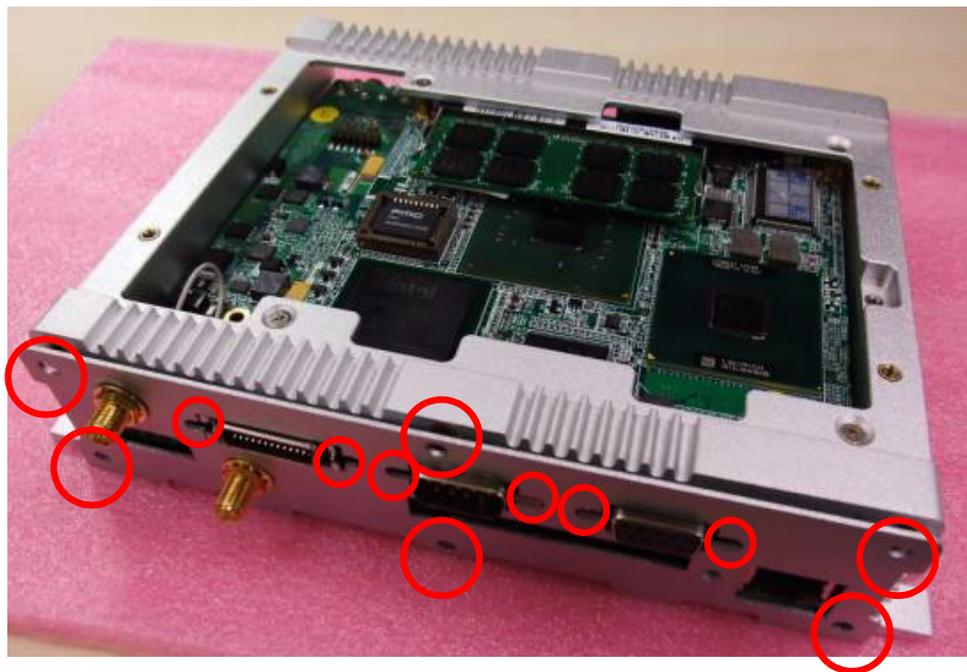
4. Assemble the front panel and note that the SMA cable is already fixed on the plate.
