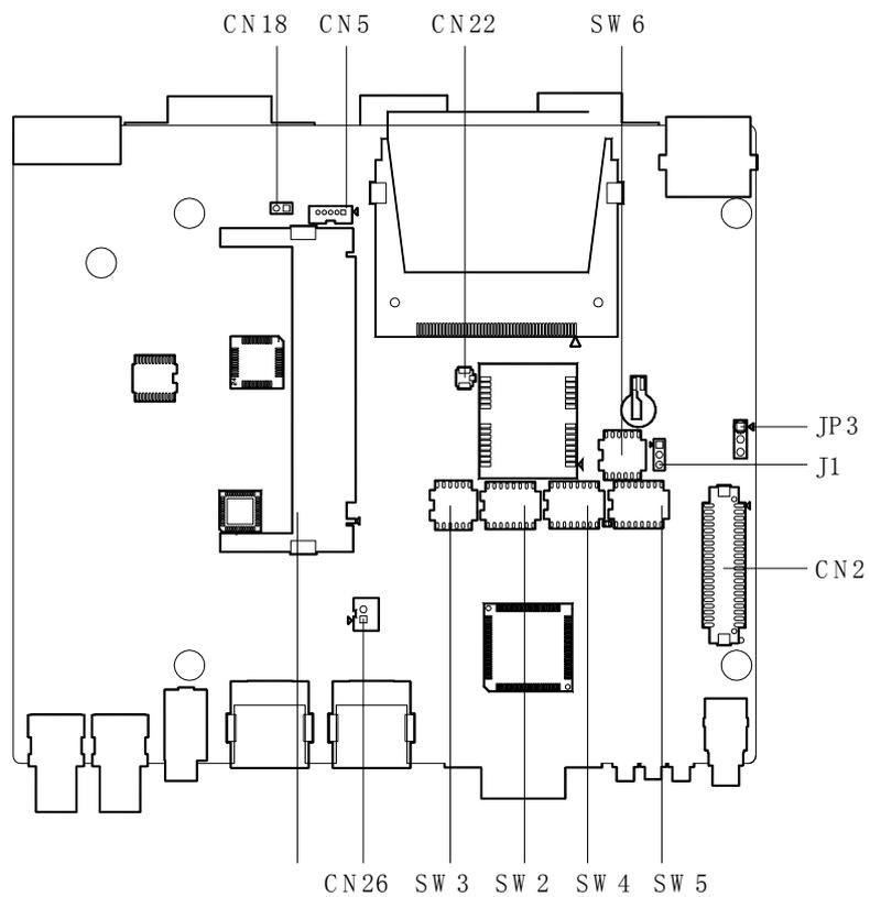
**Figure 2.2 Locating Jumpers on the Board-Bottom side**
