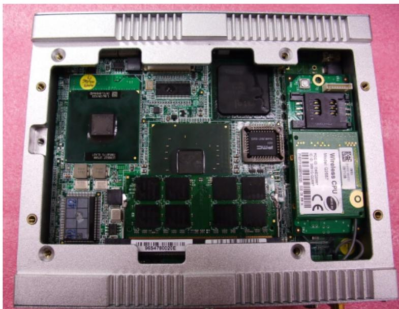
Figure 5.7 Installation AMO-EDGE on ARK-1388V
