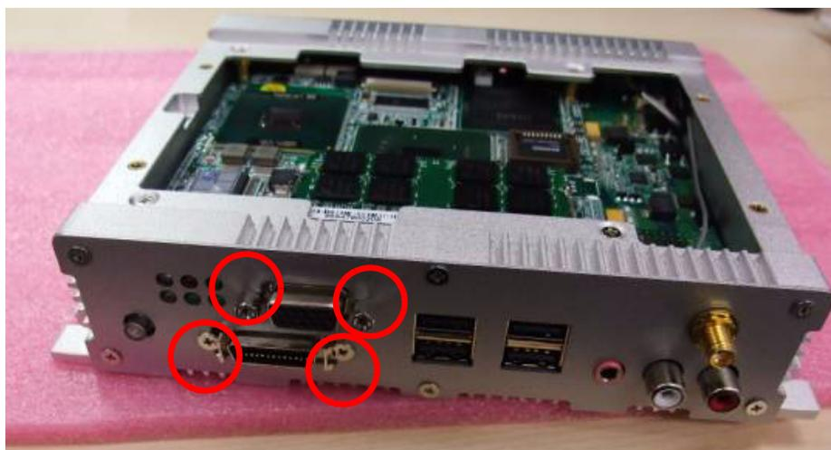
5. Please be careful take off the internal SMA Cable before taking out the front plate.
