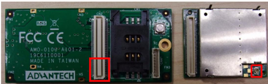
**Figure 5.3 AMO-EDGE base board and wavecom module**
