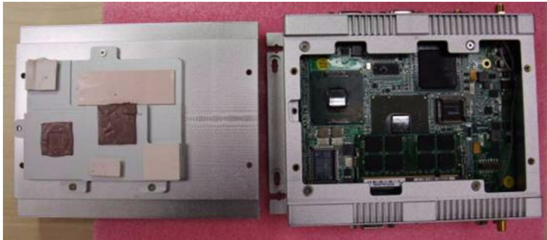
3. Unscrew the 6 screws on the front panel.
