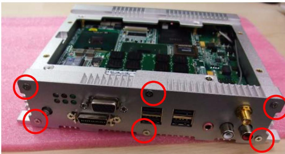
4. Unscrew the screws in the middle of the front panel
