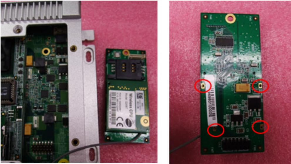
**Figure 5.6 Mounting wavecom on AMO base board**
