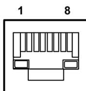
Figure 2.10 Ethernet connector
