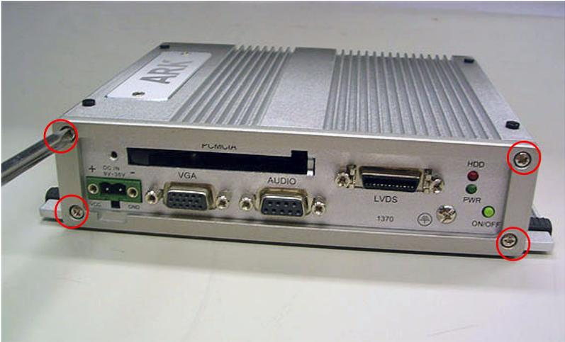
*Figure 6.5: Unscrew the 4 screws on the rear side frame*
