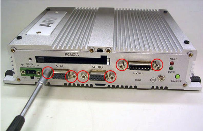
*Figure 6.7: Unscrew the 6 Hex-bolt on the rear face plate*
