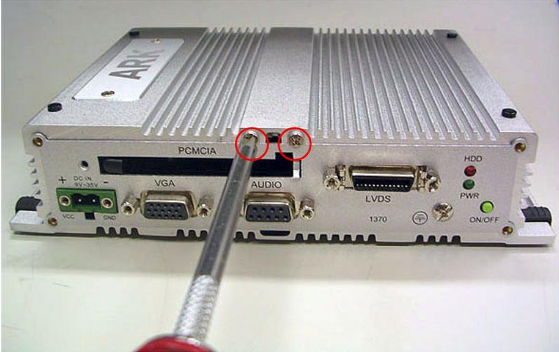
*Figure 6.6: Unscrew the 2 screws on the rear face plate*
