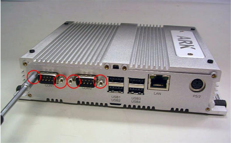
*Figure 6.4: Unscrew the 4 Hex-bolt on the front face plate*
