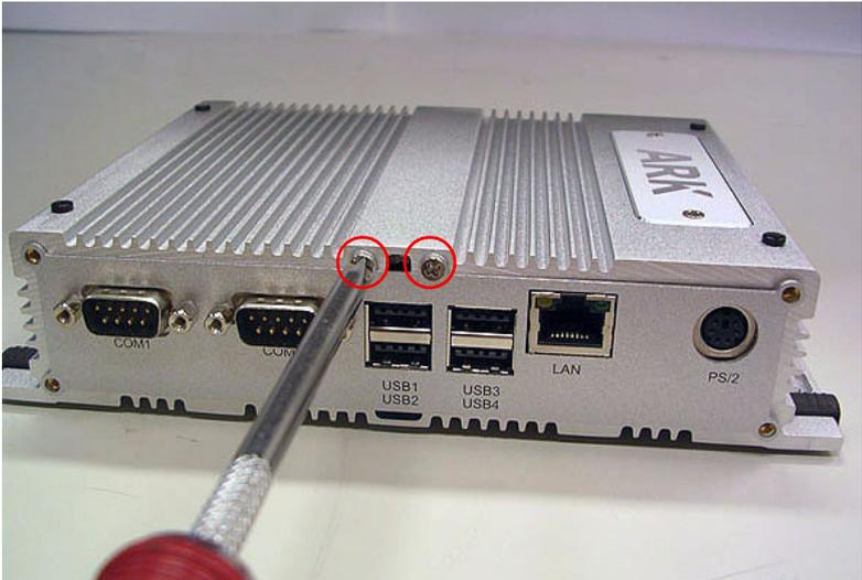
*Figure 6.3: Unscrew the 2 screws on the front face plate*
