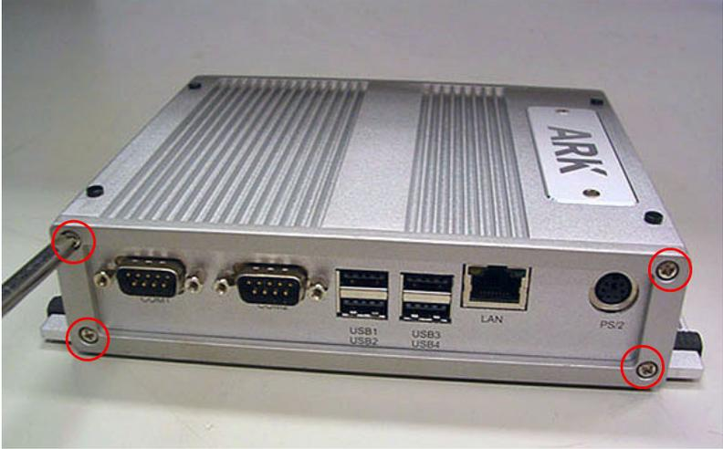
*Figure 6.2: Unscrew the 4 screws on the front side frame*
