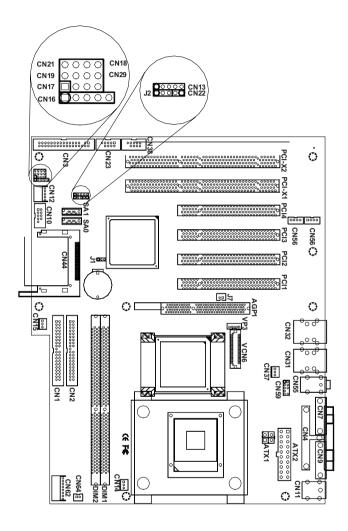
**Board Layout: Jumper and Connector Locations**
