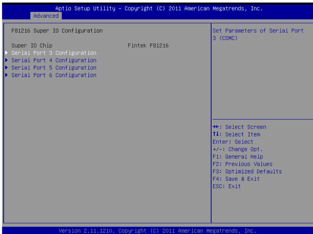
AIMB-581QG2 version supports 2nd super IO for COM 3-6, so this page of the BIOS menu is to set respective serial port configuration.
