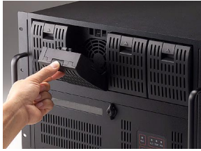
Figure 2.18: System H/S Cooling Fans
