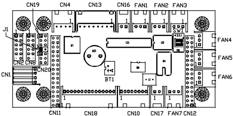
Figure 3-1: Alarm Board Layout
