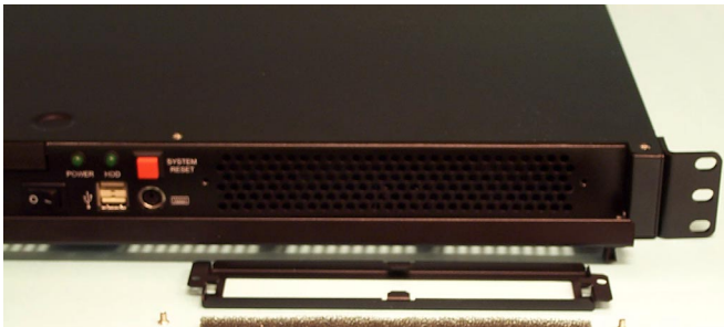
Figure 2.22: Replacement of filter
