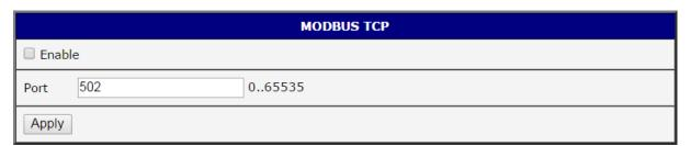
Figure 4: Modbus TCP configuration
