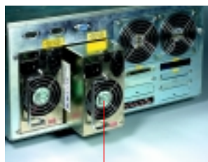
Redundant Power Supply
