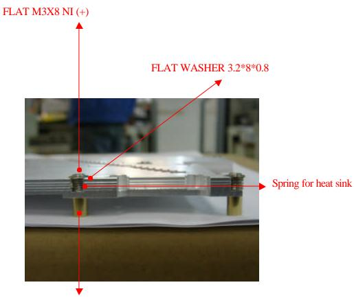
heat sink copper post for MIC-3377 A1
