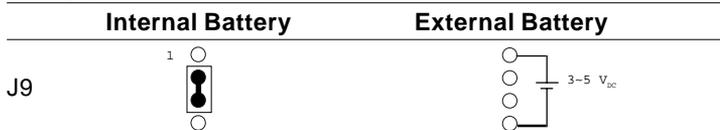
Note: You must apply battery when using SRAM
